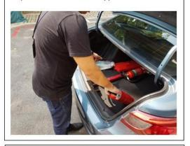
Step 4: Remove the Safety pin and squeeze the handle fully till engine fire is put out
