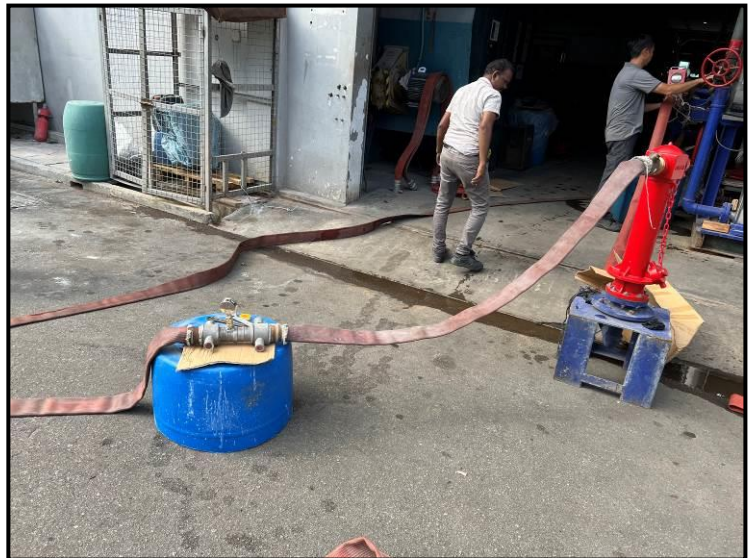
Photograph 2 shows Pillar Hydrant under Flow Characteristic Test
