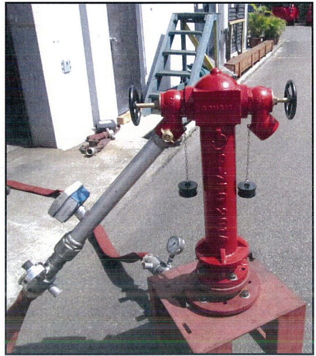
Photograph 2 shows Pillar Hydrant under Flow Characteristic Test
